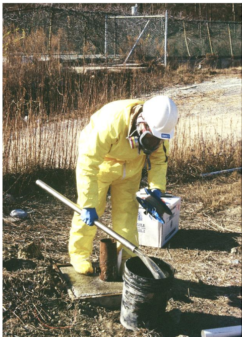
Figure 15.7 Purging a monitoring well with a bailer before collecting sample for laboratory analysis.
