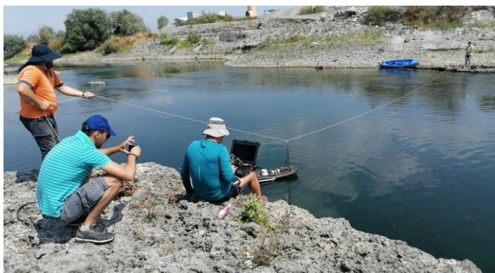
Figure 15.9 Doppler radar hydrometry of a river in karst. Following the rope extended between two river sides doppler collects and calculates information on riverbed depth and water velocity. Such hydrometry is essential method to estimate hidden water losses or inflows along the river. Courtesy of Zoran Stevanović.
