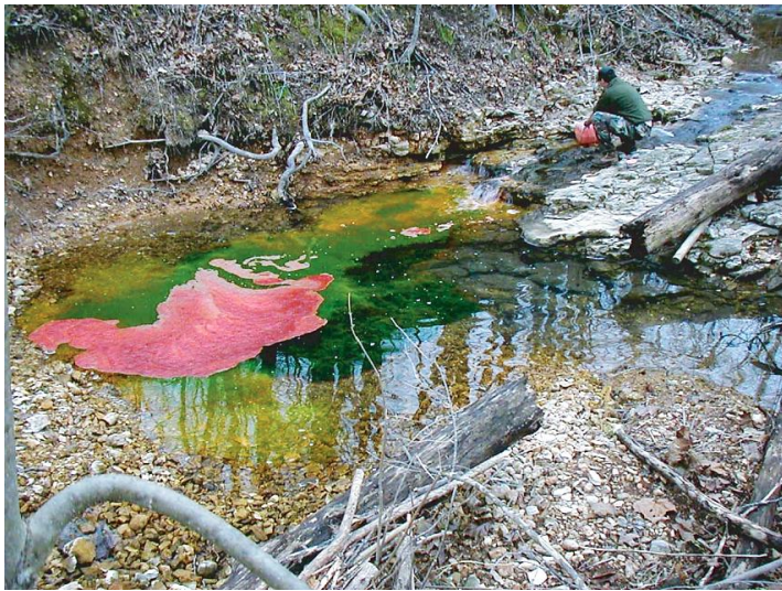
Figure 15.41 Injection of eosine OJ dye into a swallow hole in the Hughes Spring area. Photograph by Jaysson Funkhouser, USGS. From Galloway, 2004. USGS, in public domain.
