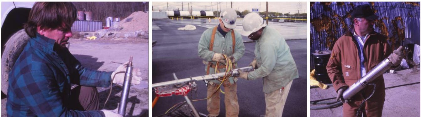
Figure 16.31 Submersible well pumps come in many different sizes and capacity, from gallons per minute to tens of gallons per minute (shown on the photos), and as powerful as hundreds of gallons per minute or more, with the lift of hundreds of feet or more.
