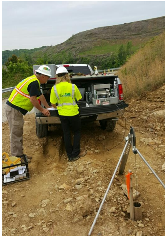
Figure 14.18 Geophysical borehole logging setup. Photo courtesy of Dawit Yifru.
