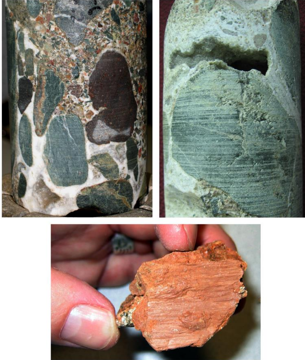
Figure 6.18 Rock core samples collected from a fault zone in aquifer developed in semi-consolidated Quaternary sediments near Phoenix Arizona (core diameter approximately 6 cm). Top left photo depicts conglomerate clasts vertically oriented along their long axis, likely a post depositional deformational feature. Top right photo illustrates potential groundwater circulation pathways through sediments partially cemented with calcium carbonate. Bottom photo depicts clear evidence of brittle deformation (faulting) with the observation of slickensides within the rock core. The cores are from borings completed in sediments routinely described as “sand and gravel” by water supply well drillers and in various published reports. Courtesy of Jeff Manuszak.
