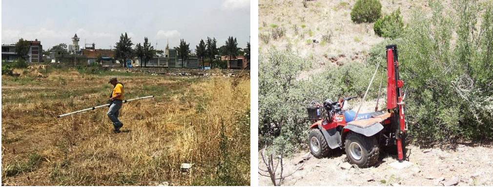
Figure 14.2 Left : Electromagnetic survey (EM) with terrain conductivity meter (antenna). Photo courtesy of Jeff Manuszak. Right : Shallow seismic reflection survey using light ATV mounted Accelerated Weight Drop in rugged terrain. Photo courtesy of Finn B. Michelsen.
