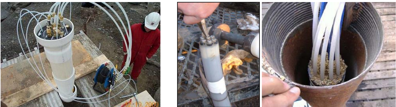
Figure 14.27 Examples of commercially available multi-level monitoring systems. Left photo: FLUTe, Flexible Liner Underground Technologies ( https://www.flut.com/ ). Two right photos: single-casing Multilevel Groundwater Monitoring System CMT by Solinst ( https://www.solinst.com/products/multilevel-systems-and-remediation/ ). All photos courtesy of Peter Thompson.
