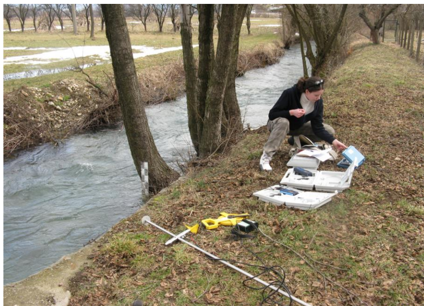
Figure 15.6 Monitoring spring water quality. Field equipment includes probes for measuring electrical conductivity, pH, water temperature, redox potential (ORP), and turbidity. Note a flow measurement device in the front. Courtesy of Zoran Stevanović.
