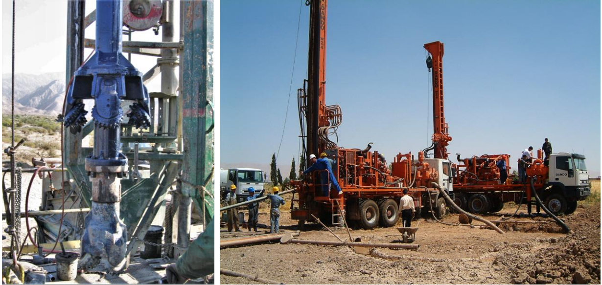
Figure 16.21 Left : Combined roller cone bit in two stages for drilling deep, large-diameter production wells. Photo courtesy of Adrian Ezeagy. Right : Drilling rigs in operation in northern Iraq (Kurdistan Province). The combined rotary and down-the-hole hammer (DTH) techniques are applied to drill formations of unconsolidated topsoil and clay, and underlying limestone. Groundwater depth in this arid region is regularly below 50 meters, but a karst aquifer could be highly productive resulting at certain points with well yields exceeding 50 L/s. Courtesy of Zoran Stevanović.
