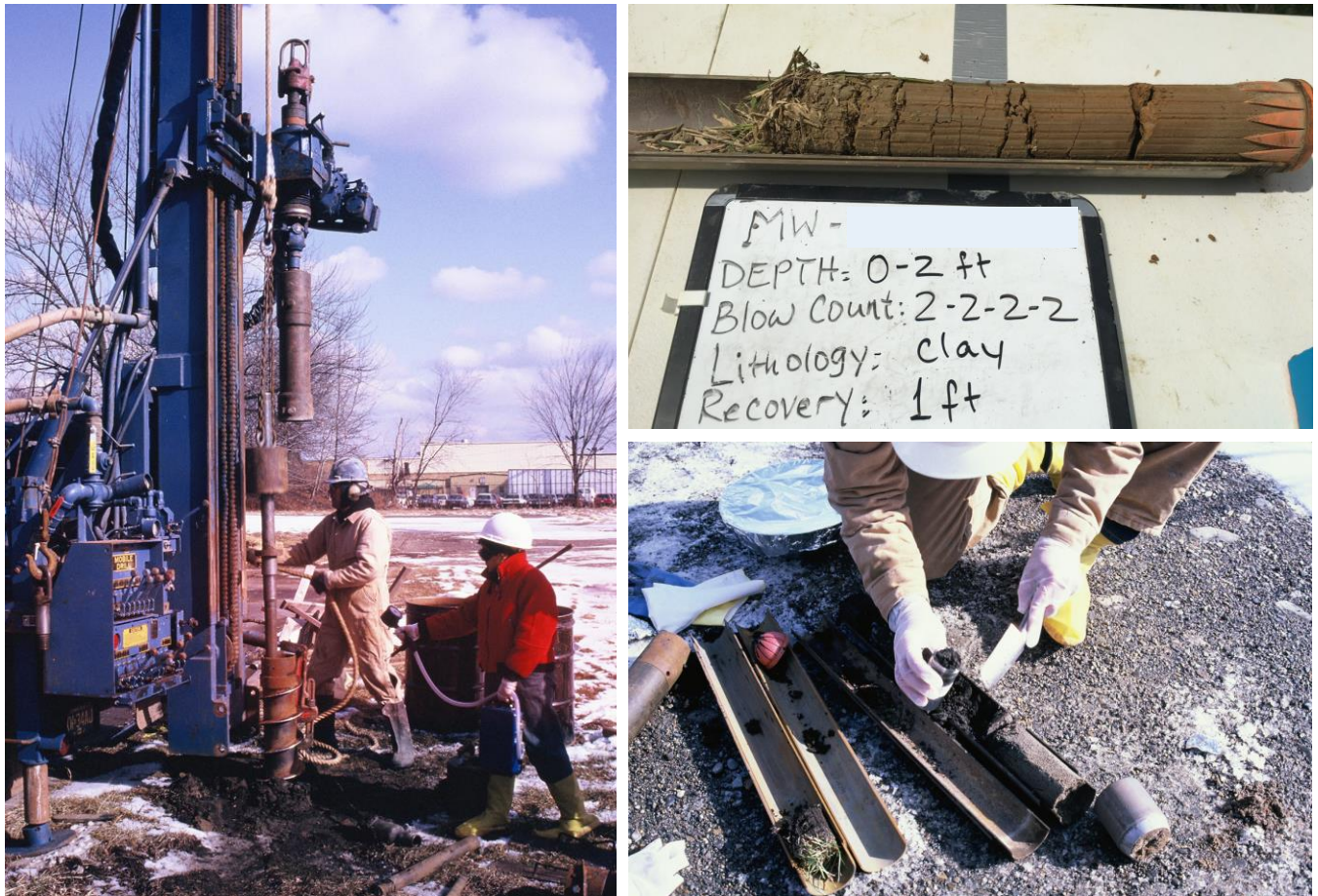
Figure 14.9 Left: Driving (hammering) split-spoon sampler through hollow-stem auger. Right: soil samples are exposed after retrieving and splitting the sampler. Bottom right photo shows collection of hydrocarbon-contaminated soil sample for laboratory analysis. Top right photo courtesy of Dawit Yifru.
