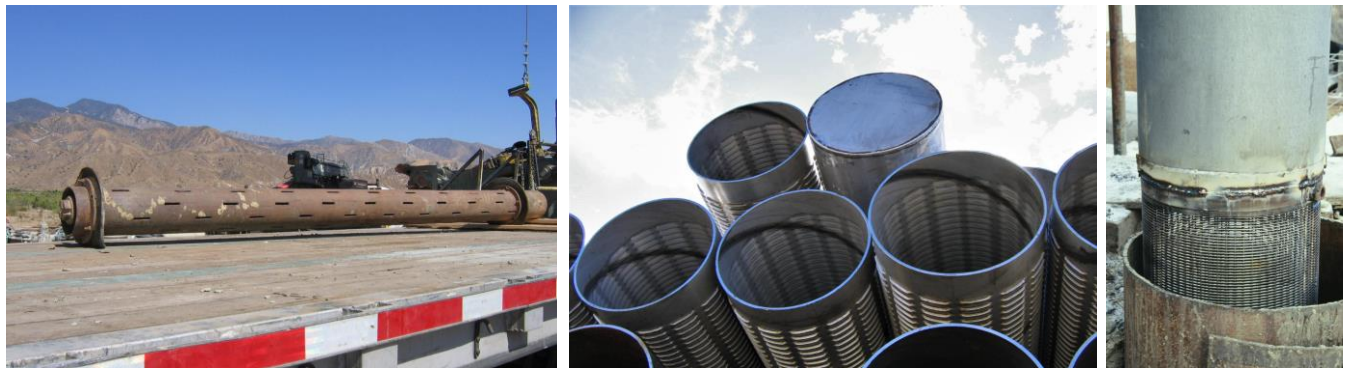
Figure 16.24 Common types of screens for high-capacity production wells. Left: Slotted casing, photo courtesy of Adrian Ezeagy. Middle: Shutter type screen, photo courtesy of Adrian Ezeagy. Right: Continuous slot wire-wound stainless-steel screen (often referred to as Johnson screen) welded to the riser pipe and being lowered into a newly drilled well.
