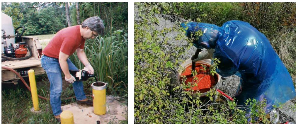
Figure 15.39 Left: Injection of Rhodamine WT into a water-level observation well. Photo courtesy of Charles J. Taylor, USGS. Right: Dilution of sodium fluoresceine prepared for dye tracing experiment in karst. Dilution of powdered tracer is with water, but use of NaOH and/or alcohol may accelerate the process. Courtesy of Zoran Stevanović.
