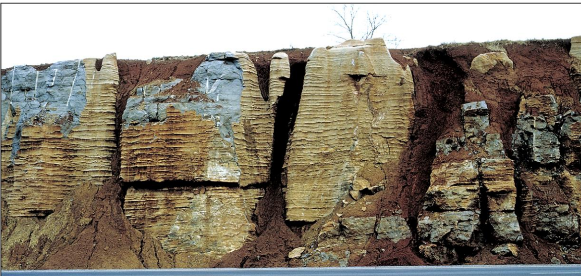
Figure 7.34 Highly weathered and karstified carbonates (“epikarst”) in a road cut near Knoxville, Tennessee. Photo by George Sowers, printed with kind permission of Francis Sowers.
