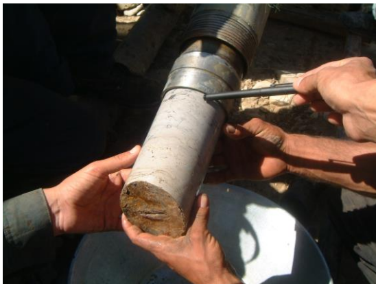
Figure 14.16 Core sample of compact limestone taken by wire line technique. Courtesy of Zoran Stevanović.
