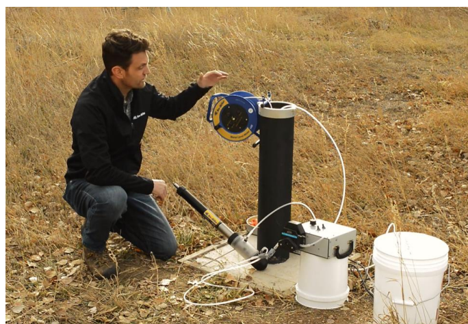
Figure 15.8 Left : Low-flow sampling equipment. Courtesy of In-Situ ( https://in-situ.com/us/low-flow-sampling ). Right : Low-flow sampling at a site in Pennsylvania, U.S. Photo courtesy of Jeff Manuszak.
