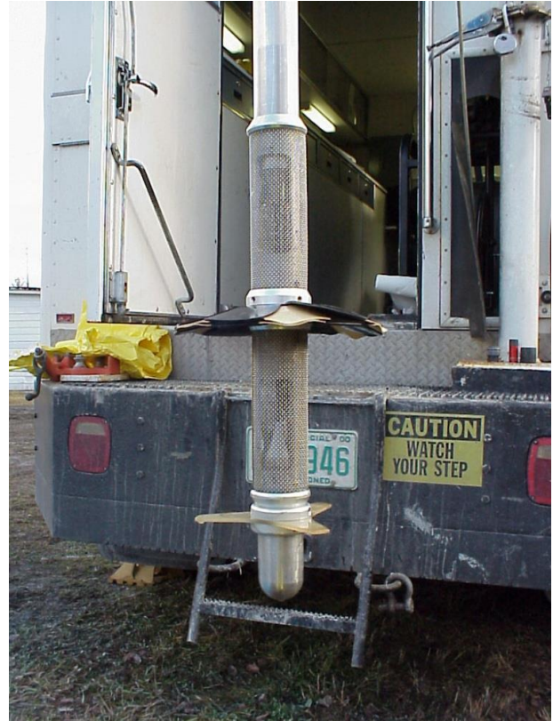
Figure 15.24 Left : Graph of ambient vs. pumping flow rates at discrete intervals in an open bedrock borehole. Right : Heat Pulse Flow Meter for characterization of fracture-specific groundwater flows in open bedrock boreholes under ambient and pumping conditions (shallow pump intake ~ 20 ft pumping at +0.1 gpm). Right : Graph of ambient vs. pumping flow rates at discrete intervals in an open bedrock borehole. Courtesy of Peter Thompson and Scott Culkin.
