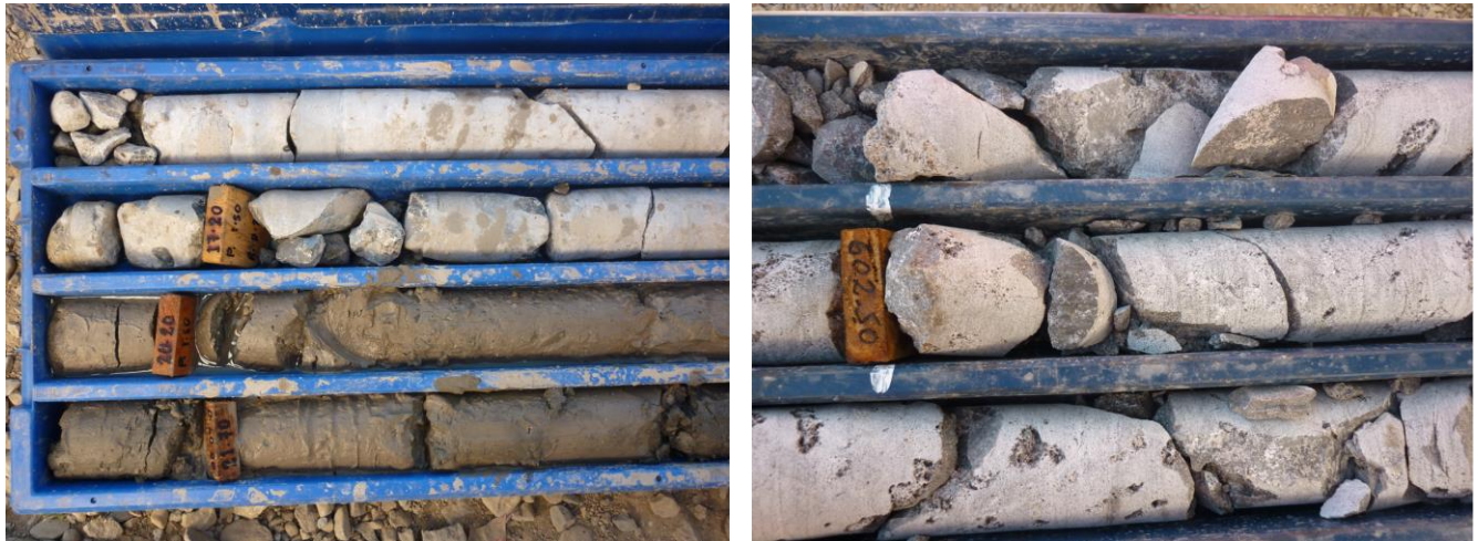
Figure 14.17 Dolomitic rock core from deep exploration boring at a site in Peruvian Andes. Left: Upper, highly weathered portion of bedrock with a clay-filled cavity. Right: Broken-up core in highly fractured and karstified (vuggy) section of bedrock at ~600 meters (1,970 feet) below ground surface.
