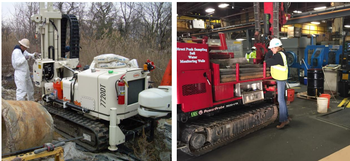
Figure 14.10 DPT rigs are small, maneuverable, and easily adaptable to various drilling conditions including in closed spaces. Left photo courtesy of Jeff Manuszak, right photo courtesy of Nick McMillan.
