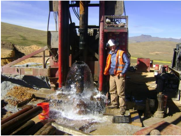
Figure 16.22 This powerful rotary drill rig encountered an artesian water-bearing horizon at depth exceeding 400m (1,300 ft), Peru. Photo Courtesy of Dave Evans.
