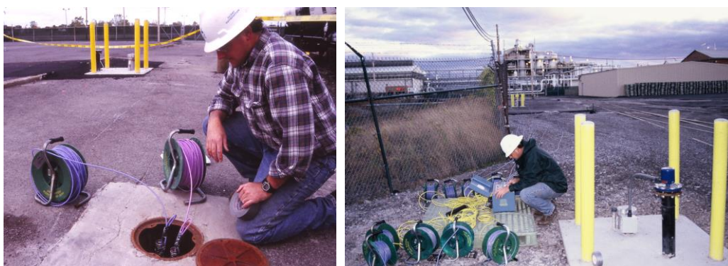
Figure 15.27 Hydrogeologist Andy Clark of Law Engineering and Environmental Services setting up a system for continuous monitoring of multiple monitoring wells at the startup of a pump-and-treat groundwater remediation at a site in New England. Cables from pressure transducers at the wells converge on the central datalogger. The site is paved, and many wells are flush mounted, which is necessary at operational industrial facilities with traffic.
