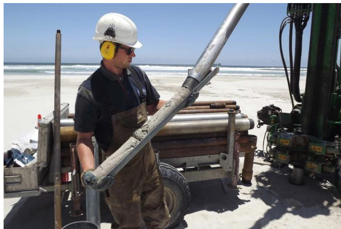
The flexibility of advancing a temporary outer casing as the borehole is drilled minimizes the risk of cross contamination. More information on sonic drilling and sampling can be found at https://www.boartlongyear.com/insite/sonic-drilling-works/
