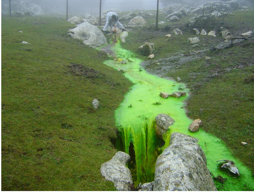
Figure 5.37 Dye tracing test with uranine in the karst system of Alta Cadena range near Malaga, Spain. Courtesy of Bartolome Andre Navarro, CEHIUMA.
