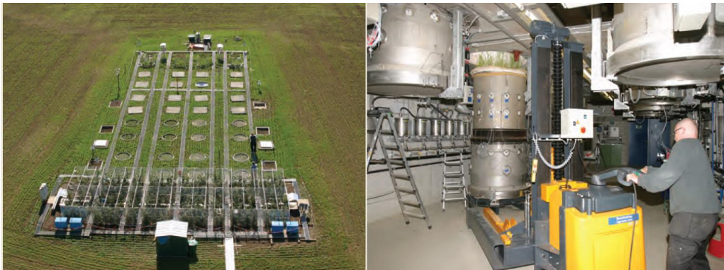
Figure 8.27 Left : Array of lysimeters operated by Helmholtz Center Munich, Germany. Right : Below-ground view of one of the lysimeters. Photographs courtesy of Dr. Sascha Reth.
