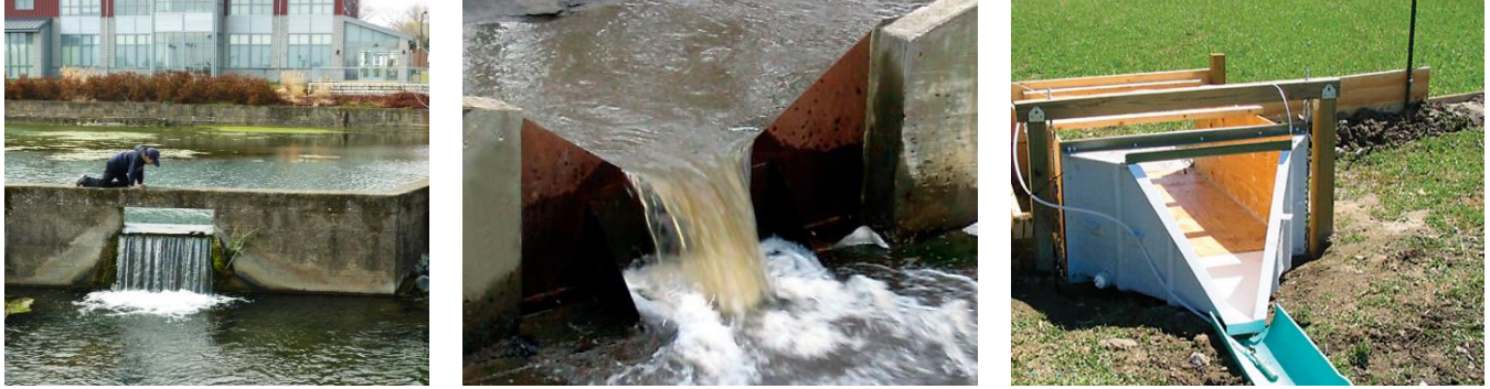
Figure 15.11 Left : Rectangular weir measuring outflow from a spring in Winchester, Virginia formerly utilized for public water supply. Middle : Sharp-crested 120 degrees V-notch weir. Right : Prefabricated H flume. Two right photographs courtesy of Don Meals, Tetra Tech, Inc., from NNPSMP, 2008; in public domain.
