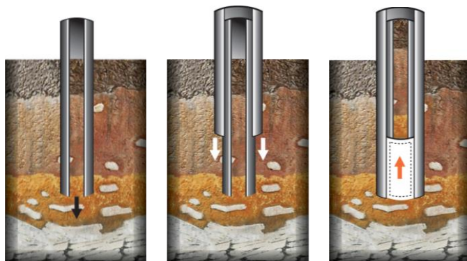
Figure 14.12 The sonic drilling procedure. Step 1 (left): The core barrel is advanced using sonic frequencies. When necessary this step can be performed using no fluids, air, or mud. Step 2 (middle): After the core barrel is in place, casing is sonically advanced over the core barrel, protecting the bore hole's integrity in loose unconsolidated ground, i.e., preventing collapse. Step 3 (right): The core barrel is retrieved, producing a relatively undisturbed sample with near 100% core recovery. Steps 1 through 3 are repeated to depth. Courtesy of Fred Hafner, Boart Longyear™
