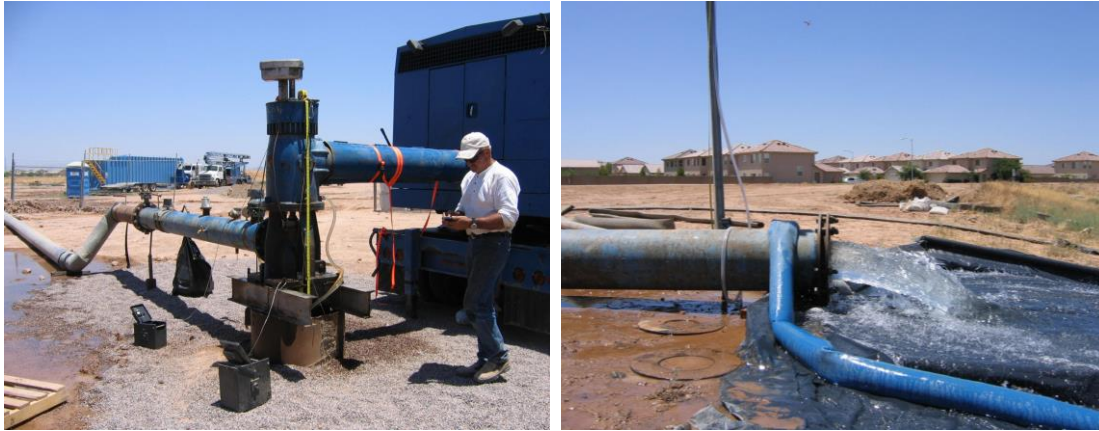
Figure 15.37 Large capacity deep production well in Arizona being tested with the maximum feasible pumping rate. Tests like this produce large quantities of water which must be managed for extended period of time, including preventing the water to circle back to the aquifer and bias the test results. Photos courtesy of Chris Legg.
