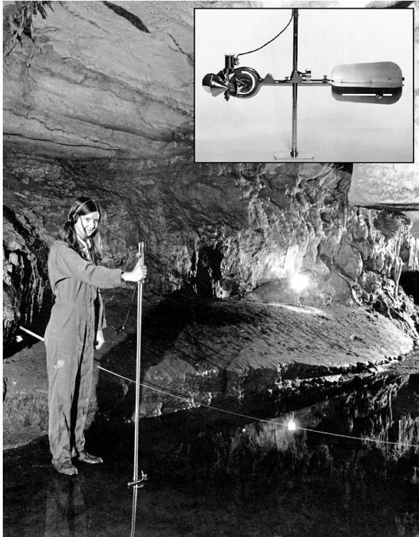
Figure 15.13 Measurement of underground flow with Price-Pigmy meter and wading rod. (Photograph courtesy of William Jones, Karst Waters Institute.) Inset: Price AA current meter on a round wading rod.
