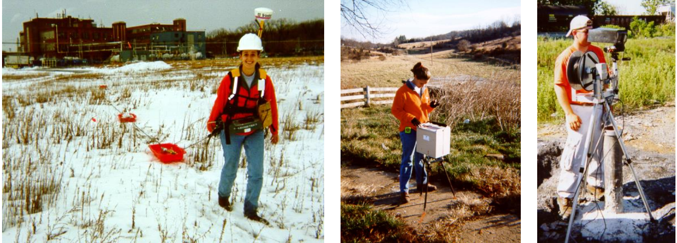
Figure 14.4 Left : Surveying with Geometrics Ohm mapper capacitively coupled resistivity meter. Middle : Scintrex CG-3M microgravity meter. Right : Borehole video inspection setup. Photos courtesy of Timothy Bechtel.
