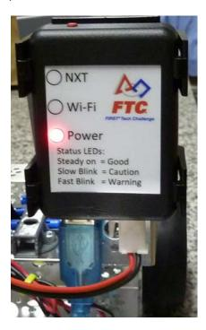
It has a usb port that connects with the NXT brick and a power port that hooks to that big battery pack you received with your kit.
