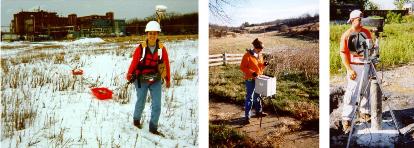
Figure 14.4 *Left*: Surveying with Geometrics Ohm mapper capacitively coupled resistivity meter. *Middle*: Scintrex CG-3M microgravity meter. *Right*: Borehole video inspection setup. Photos courtesy of Timothy Bechtel.
