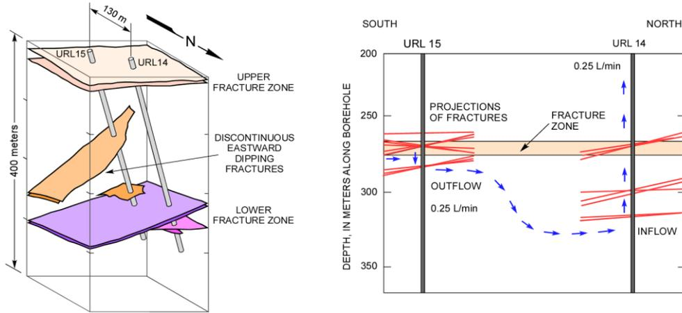
Figure 5.6 *Left*: Diagram showing orientation of fractures intersecting boreholes URL14 and URL15 determined from acoustic televiewer logs and projections of fractures between the two boreholes. *Right*: Diagram showing inferred hydraulic connection between boreholes URL14 and URL15 during crosshole pumping tests. Modified from Paillet, 1989. USGS, in public domain.
