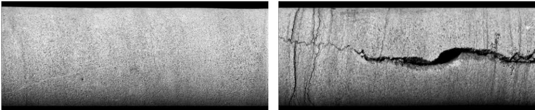
Figure 7.17 Two core samples from the same boring in Ordovician Lexington Limestone near Lexington, Kentucky. Core diameter is 4.5 cm (approximately 2 in.)
