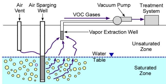
Figure 13.20 Illustration of a combined air sparging and SVE system. Modified from U.S. EPA 1996a, in public domain.
