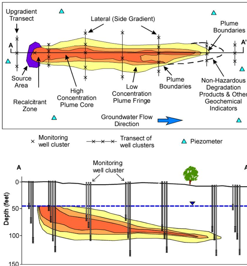
Figure 14.21 Example of a monitoring well network at a groundwater contamination site. *Top*: map view. *Bottom*: Cross-sectional view. From Ford et al., 2007; U.S. EPA, in public domain.
