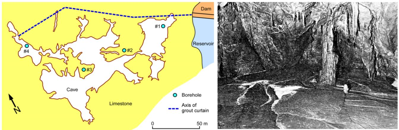
Figure 7.16 *Left*: Cave in the left abutment of Sklope Dam, Croatia discovered with an exploration gallery which was excavated after extensive grouting failed to achieve backpressure. *Right*: The grout mass on the cave floor. Modified from Božičević, 1971; photo courtesy of Srećko Božičević.
