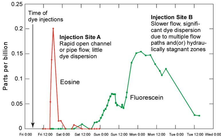
Figure 15.42 Example of dye-breakthrough curves for two dye-tracing tests conducted in the Edwards aquifer, Texas, showing a quick-flow response with little or no dispersion (Injection site A, left), and a slow-flow response showing the effects of dye dispersion (Injection site B, right). Courtesy of Geary Schindel, Edwards Aquifer Authority; from Taylor and Green, 2008. USGS, in public domain.
