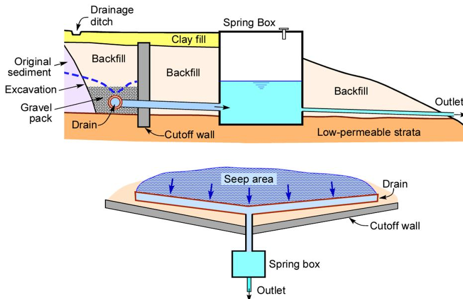
Figure 16.32 Capture of a seepage spring. *Top*: Cross-sectional view. *Bottom*: Plan view. Modified from Jennings, 1996; North Carolina Cooperative Extension Service; in public domain.
