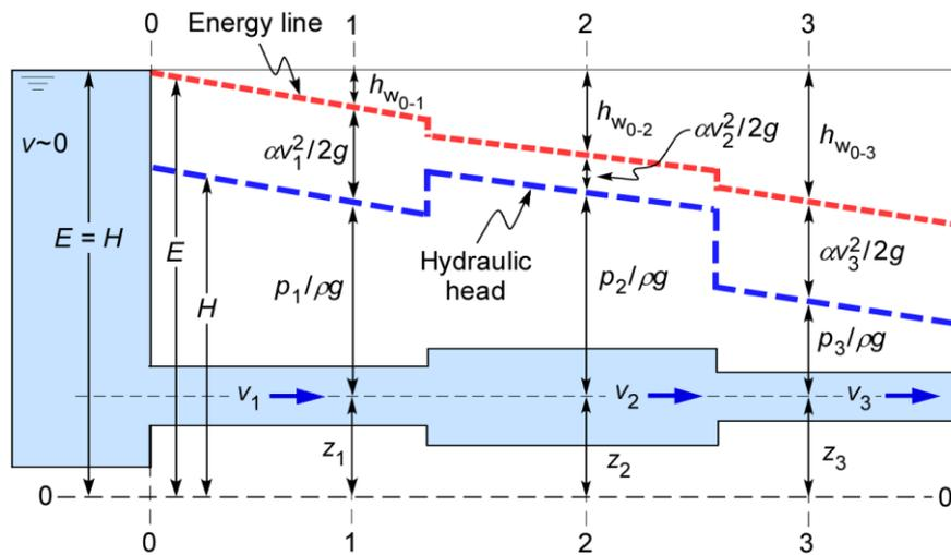
Figure 5.14 Illustration of the Bernoulli equation for flow of real viscous fluids through a pipe with the varying cross-sectional area. Energy line ( $E$ ) at any given cross-section is the sum of the elevation head ( $z$ ), the fluid pressure head ( $p/\rho g$ ) and the velocity head ( $\alpha v^2/2g$ ). The fluid pressure head and the elevation head give the hydraulic head—see Equation (5.10) Modified from Kresic, 2013. Copyright McGraw Hill; permission is required for further use.
