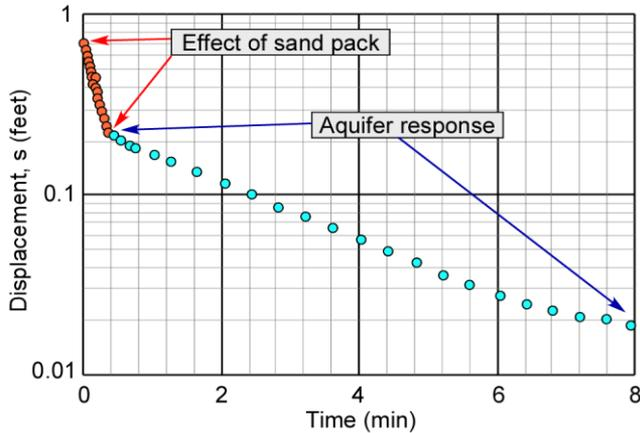
Figure 15.21 Example graph time vs. head displacement (s) for a falling head slug test.
