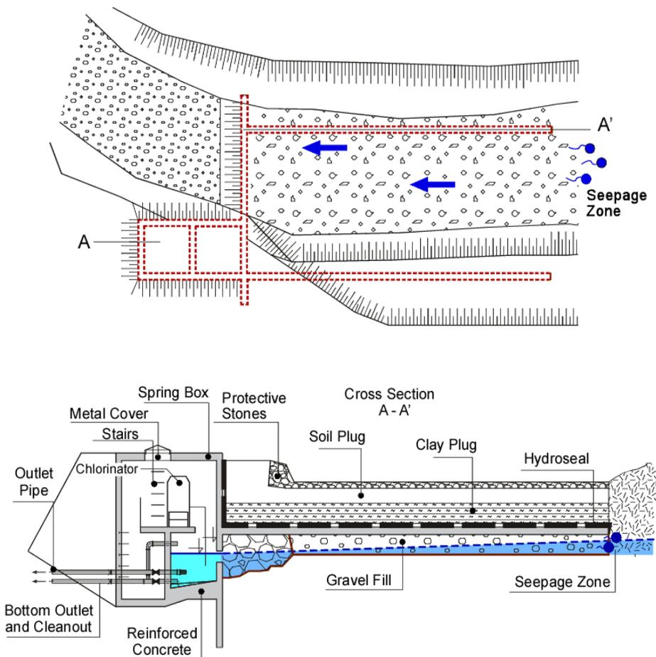
Figure 16.33 Capture design of a group of three seepage springs in an alluvial valley. *Top*: Map view of the excavation with the outline of the engineered structure (red dashed lines). *Bottom*: Cross-section of the spring capture. Courtesy of WIGA, Belgrade; design by Gaon, 1975; Copyright Hidroprojekt, Belgrade; permission is required for further use.
