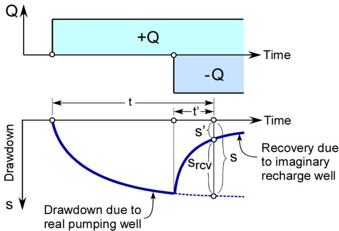
Figure 15.35 The principle of superposition of flows used to simulate the drawdown recovery during a well pumping test. Modified from Kresic, 2007. Copyright CRC Taylor & Francis; permission is required for further use.
