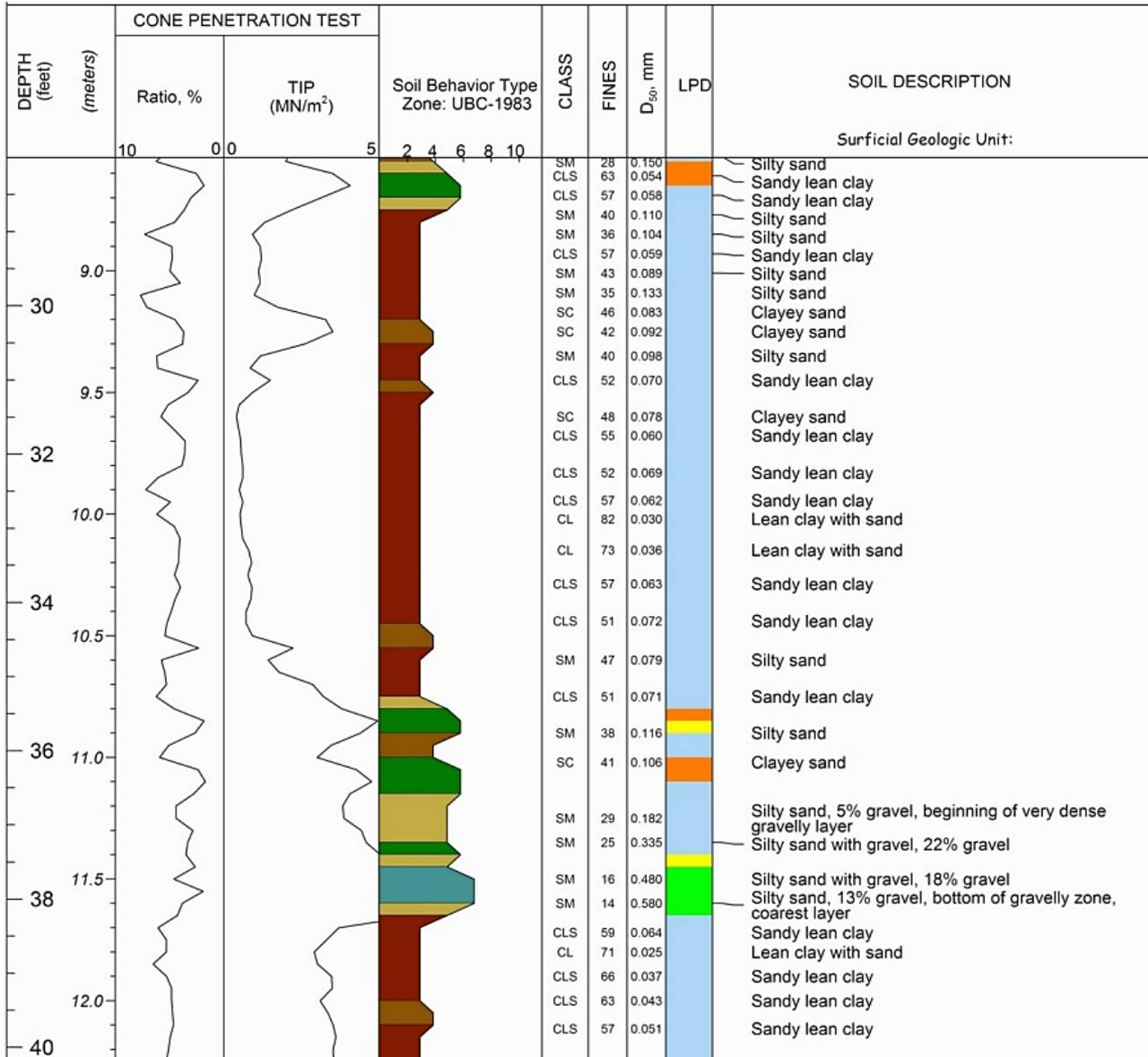
Figure 14.11 CPT log of a boring SNC007c showing tip resistance, friction ratio, UBC soil behavior type, and liquefaction potential display. From Bennett et al., 2011; USGS, in public domain.
