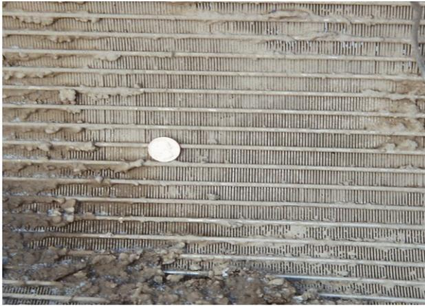
Figure 16.22 This screen was extracted from a failed production well located next to a large river in upstate New York. Because of an improper filter pack (too coarse) and screen design (openings too small), the screen became quickly completely clogged with fine silt that was interspersed with coarse glacio-fluvial sediments. The well was subsequently over-drilled and equipped with a proper screen and filter pack to prevent this from happening again. Note a coin (US quarter) for scale.
