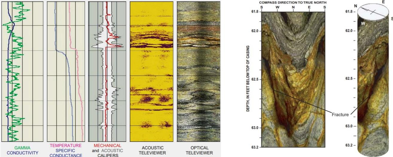
Figure 14.19 *Left*: Geophysical logs from a section of borehole MW109R, University of Connecticut landfill study area, Storrs, Connecticut. From Johnson et al., 2002; USGS, in public domain. *Right*: Optical televiwer (OTV) log of a section of borehole MW109R, as an “unrolled” 360-degree scan of the borehole wall, and “rolled” into a virtual core (right). From Johnson et al., 2002; USGS, in public domain.
