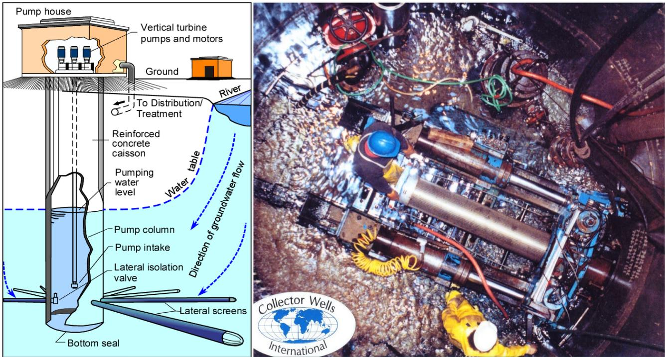
Figure 16.29 *Left*: Schematic of a typical radial collector well adjacent to riverbank. *Right*: Down view of installation of 12-inch diameter well screen in 13-foot diameter collector well. Courtesy of Collector Wells International, Inc., a Layne Christensen Company
