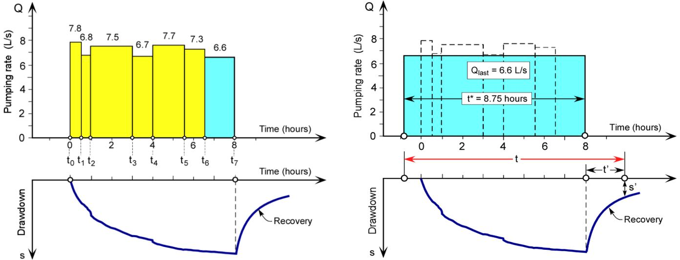
Figure 15.33 *Left*: Hydrograph of a varying pumping rate and the corresponding drawdown-recovery curve for an aquifer pumping test. *Right*: New adjusted hydrograph with the constant pumping rate of 6.6 L/s and the new time base of 8.75 hours. Note that the new beginning of the test is shifted to the left of the original startup time. Modified from Kresic, 2007. Copyright CRC Taylor & Francis; permission is required for further use.
