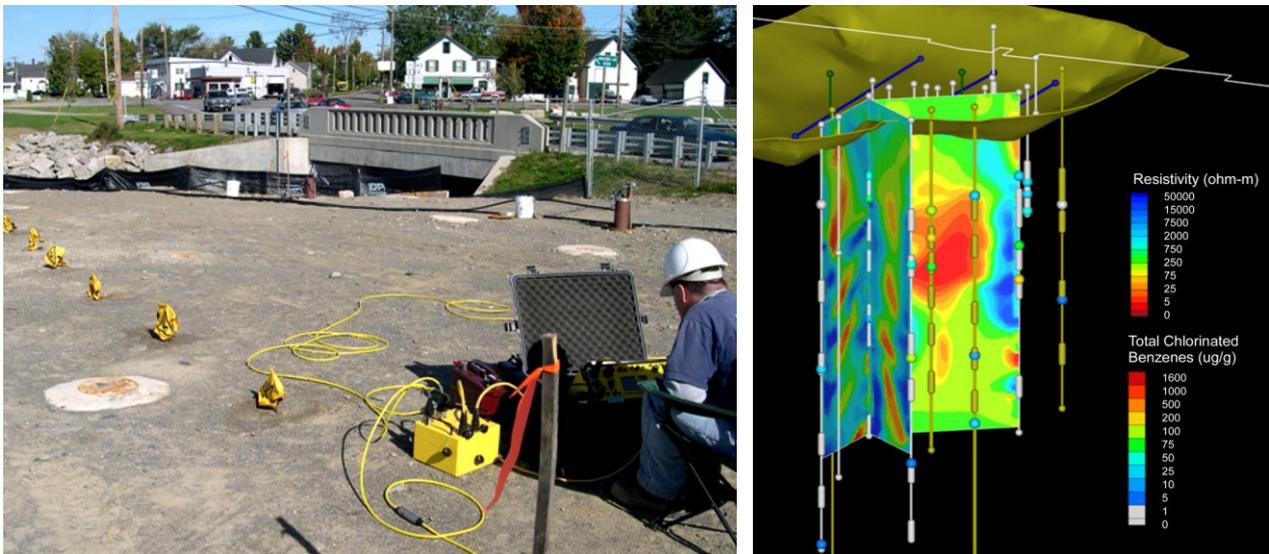
Figure 14.20 *Left*: Setup for determining presence and 3D orientation of fractures using electrical resistivity tomography between boreholes. *Right*: Electrical resistivity tomography results shown in panels between boreholes; concentration of contaminants of concern are for discrete sampling points shown as spheres. Courtesy of Peter Thompson, Scott Calkin, and Rod Rustad.
