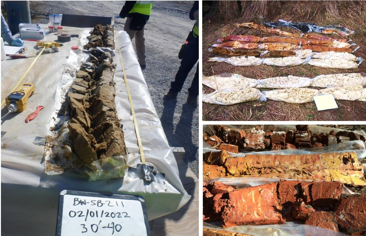
Figure 14.14 *Left*: Examining and sampling a 10-foot sonic core of silty sand retrieved in plastic sleeve. Courtesy of Nick McMillan. *Right*: Sonic cores of clay (yellow to brown color) and white “sand”. In this case, “sand” is weakly cemented Ocala limestone which lost its cohesion due to sonic drilling and can therefore be easily mischaracterized (see also Figure 5.13 in Lecture 5).
