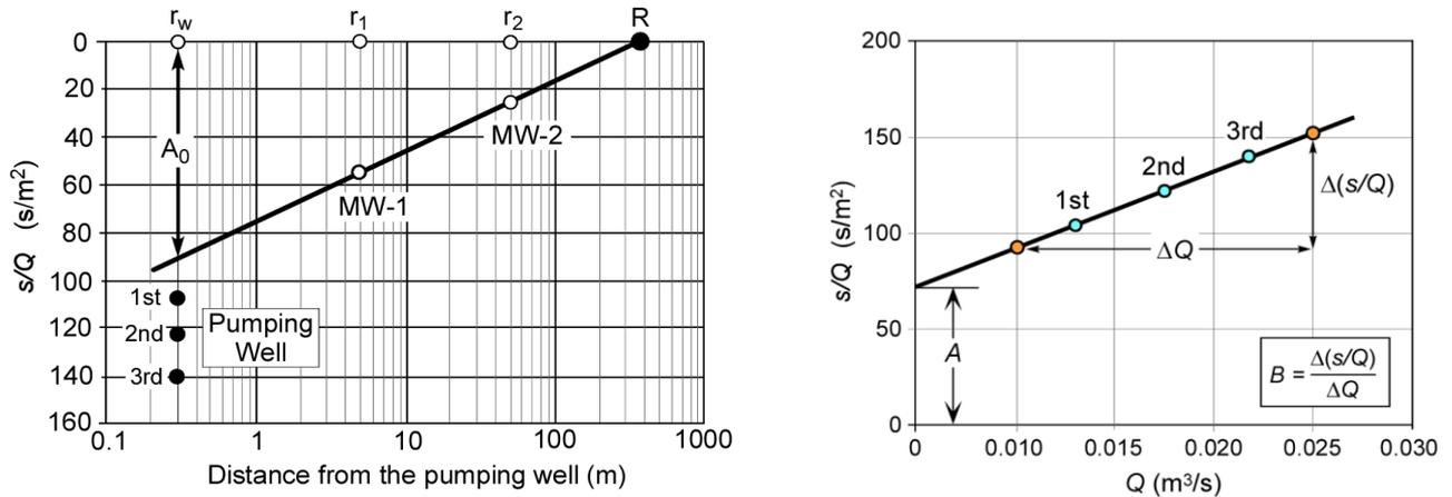
Figure 15.29 Left: Graph distance versus  $s/Q$  for three-step pumping test in quasi-steady-state conditions, showing data for pumping well and two monitoring wells. Right: Graph pumping rate ( $Q$ ) versus drawdown-pumping rate ratio ( $s/Q$ ) for a three-step well pumping test. From Kresic, 2009. Copyright McGraw Hill; permission required for further use.
