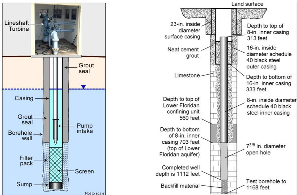
Figure 16.28 *Left*: Schematic of a typical vertical well completed in unconfined aquifer. *Right*: Well-construction diagram for well HAAF 11 (36Q392) completed in the Lower Floridan aquifer, Hunter Army Airfield, Chatham County, Georgia. Modified from Clarke et al., 2010; USGS, in public domain.
