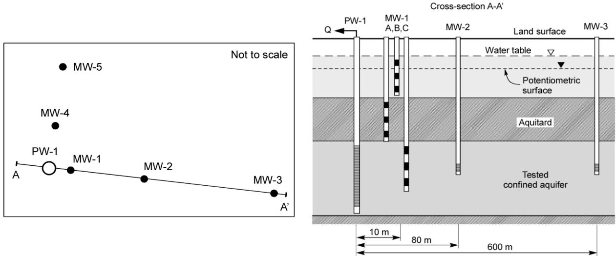
Figure 7.50 An example of a pumping test monitoring well network designed to determine characteristics and anisotropy of the tested confined aquifer, and nature of the aquitard including possible leakage from the aquitard and the unconfined aquifer into the underlying confined aquifer. PW-1: pumping well; MW-1 cluster of multiport wells; MW-2 and MW-3: single screen monitoring wells. *Left*: map view; *Right*: cross-section.
