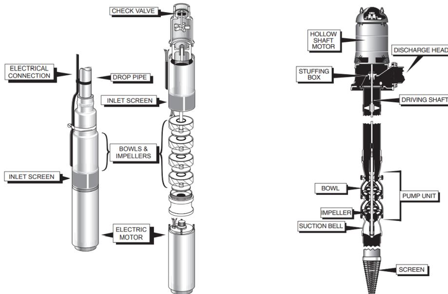
Figure 16.25 Two common types of vertical pumps for production wells. *Left:* Submersible turbine. Both the motor and the pump intake/hydraulic unit are submerged below the water level in the well. *Right:* Lineshaft turbine. The pump intake and hydraulic components are submerged, whereas the motor is located above ground, with easy access. From ATTAC, 2014.
