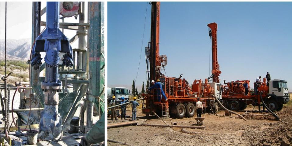
Figure 16.18 *Left*: Combined roller cone bit in two stages for drilling deep, large-diameter production wells. Photo courtesy of Adrian Ezeagy. *Right*: Drilling rigs in operation in northern Iraq (Kurdistan Province). The combined rotary and down-the-hole hammer (DTH) techniques are applied to drill formations of loose topsoil and clay, and underlying limestone. Courtesy of Zoran Stevanović.
