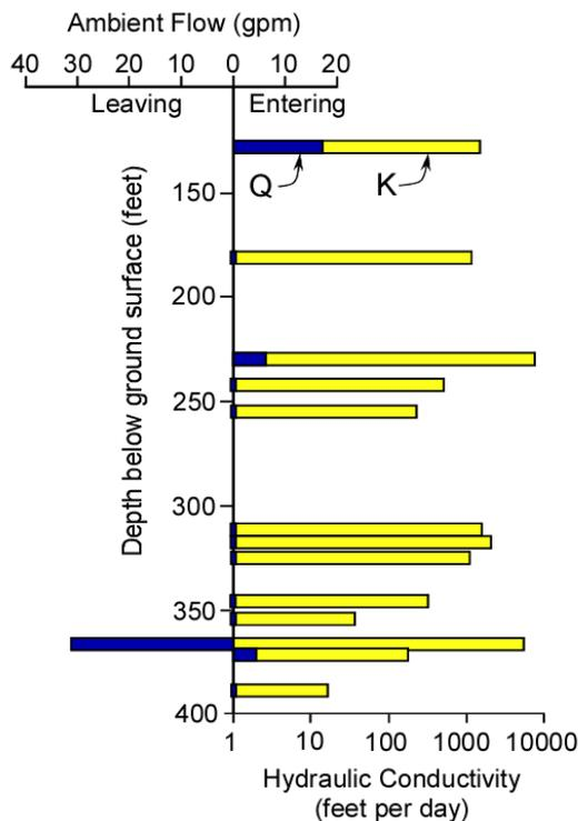
The theory of hydrophysical logging is based on the law of mass balance and the linear relation between FEC and dissolved mass. By recording the changes in the electrical conductivity in the fluid column with depth, the locations of the water-producing zones can be determined, and the volumetric rate of inflow can be calculated.
