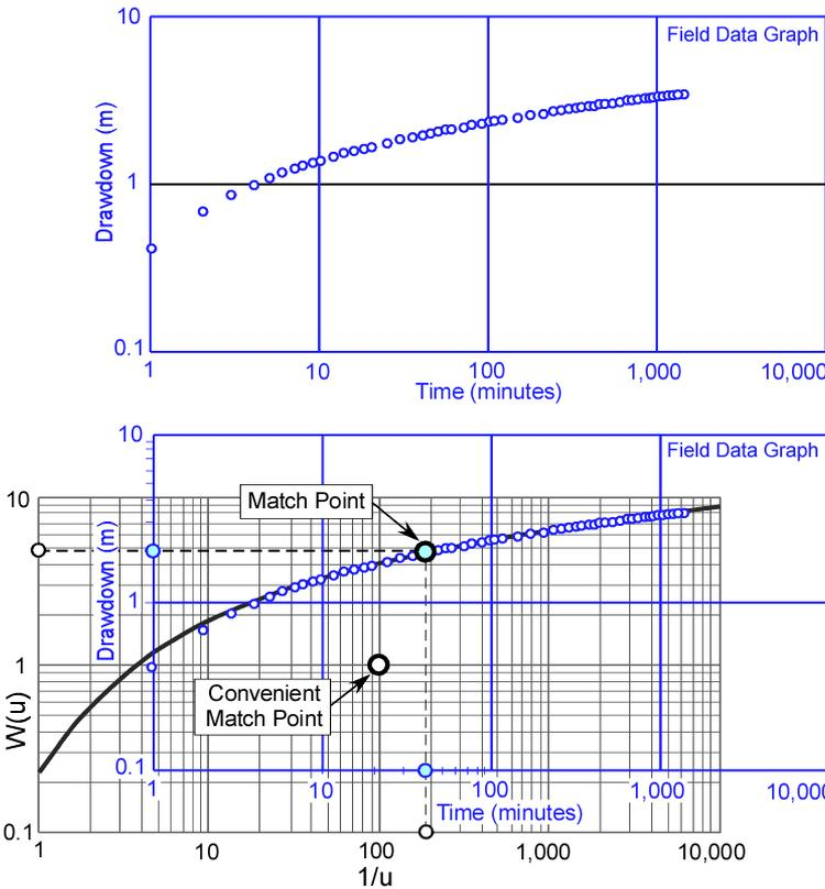
Figure 4.28 Graphoanalytical solution of the Theis equation for a pumping test data at a monitoring well located 40.5 meters from the pumping test well. The fully penetrating well was pumping from a confined aquifer for 24 hours at a constant rate of 8 liters per second (0.008 m<sup>3</sup>/s). The black graph is the theoretical Theis curve. Copyright CRC Taylor & Francis; permission is required for further use.
