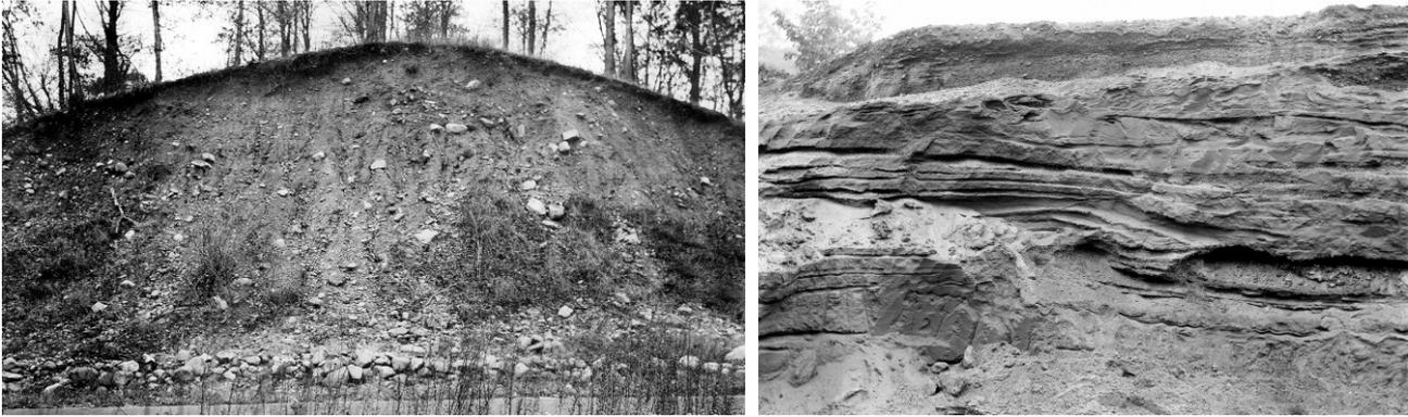
Figure 6.22 *Left*: Glacial till of the Harbor Hill terminal moraine (Wisconsin interglacial period) exposed on Long Island Motor Parkway, 1/2 mile north of Creedmoor. Hempstead quadrangle. Queens County, New York. October 29, 1917. *Right*: Stratified glacial sand and gravel, one mile north of Asticou, northeast of Lower Hadley Pond. Acadia National Park, Maine, Sep 14, 1907. Courtesy USGS Photographic Library, 2007.
