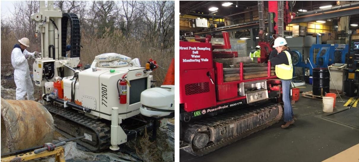
Figure 14.10 DPT rigs are small, maneuverable, and easily adaptable to various drilling conditions including in closed spaces. Left photo courtesy of Jeff Manuszak, right photo courtesy of Nick McMillan.
