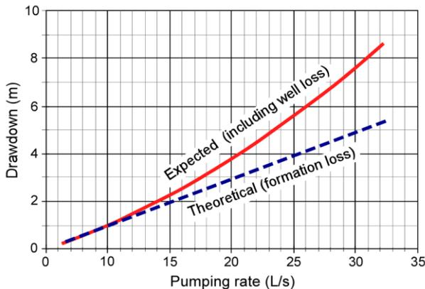
Figure 15.30 Pumping rate versus formation loss (theoretical drawdown) calculated with Equation (15.19) and the expected drawdown in the well calculated with Equation (15.17). From Kresic, 2009. Copyright McGraw Hill; permission required for further use.
