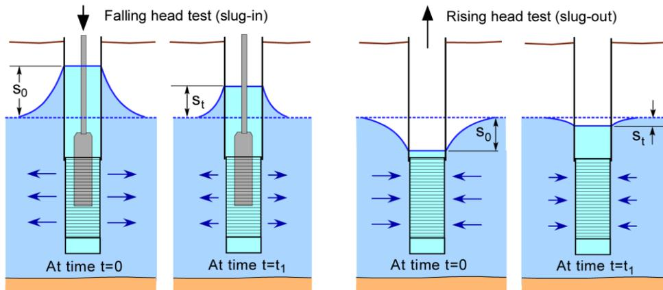
Figure 15.18 Schematic of falling head slug test (*left*), and rising head slug test (*right*). Sudden displacement from the initial water table is denoted with  $s_0$ . Modified from Kresic, 2007. Copyright CRC Taylor & Francis; permission is required for further use.
