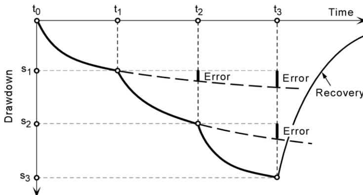
Figure 15.31 Components of drawdown recorded at the end of each step showing errors made if drawdowns  $s_1, s_2$ , and  $s_3$  were used directly to draw graph  $Q$  versus  $s/Q$ . From Kresic, 2009. Copyright McGraw Hill; permission required for further use.
