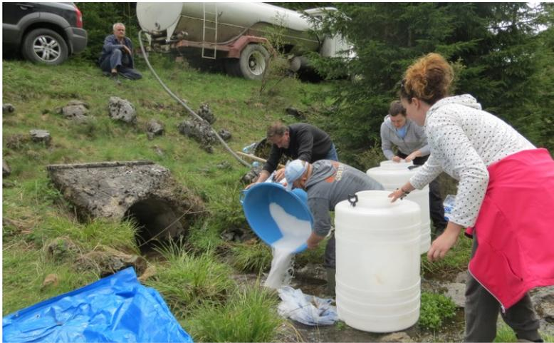
Figure 15.40 Dye tracing experiment with salt (NaCl) at one of the swallow holes in a karst aquifer of western Serbia. The water truck is used to dissolve large quantities of the tracer and chase it down the swallow hole. Courtesy of Zoran Stevanović.
