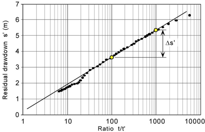
Figure 15.34 Semi-log graph residual drawdown versus  $t/t'$  ratio for determining aquifer transmissivity. From Kresic, 2007. Copyright CRC Taylor & Francis; permission is required for further use.
