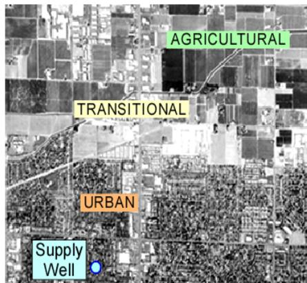
Figure 12.5 An aquifer system and public water system in an urban setting. The water entering the well screens of the public supply wells is of different ages and from different areas because of their long screen intervals, which commonly make public supply wells vulnerable to contamination from multiple sources. In this example, sources of contaminants may include those associated with urban and agricultural land use activities. Modified from Eberts et al., 2005; USGS, in public domain.
