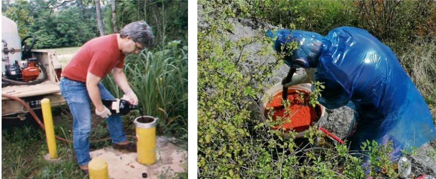
Figure 15.39 Left: Injection of Rhodamine WT into a water-level observation well. Photo courtesy of Charles J. Taylor, USGS. Right: Dilution of sodium fluoresceine prepared for dye tracing experiment in karst. Dilution of powdered tracer is with water, but use of NaOH and/or alcohol may accelerate the process. Courtesy of Zoran Stevanović.
