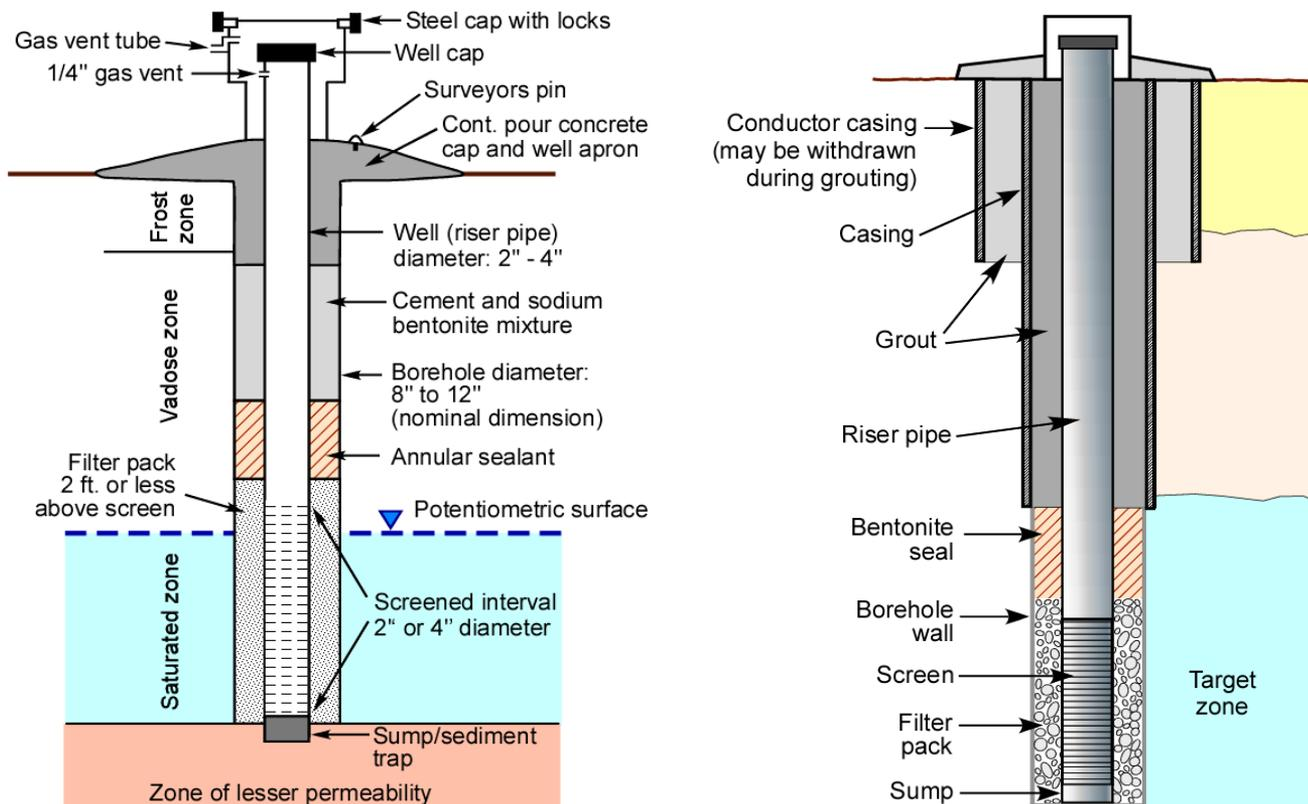
Figure 14.22 *Left*: Typical design of a standard monitoring well. Modified from U.S. EPA, 1986.
