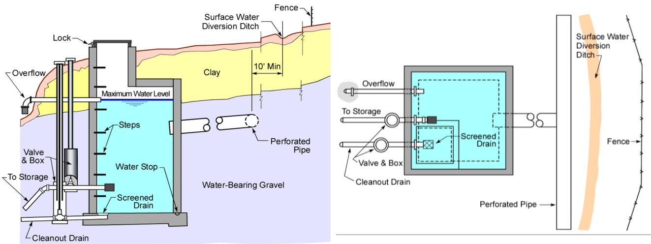
Figure 16.31 Typical capture of a gravity spring using spring box. *Left:* Cross-sectional view. *Right:* Plan view. Modified from U.S EPA, 1991; in public domain.
