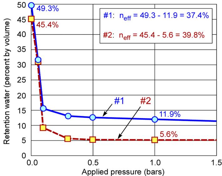
Figure 2.9 Typical graph of a water retention test by ASTM D2325, for two clean uniform beach sands. The *effective drainage porosity* is found for an applied pressure by subtracting the retained percent water (by volume) from the full saturation percent water. Applied pressure of 1 bar corresponds to free gravity drainage. From Kresic, 1998. Copyright Law Engineering and Environmental Services.
