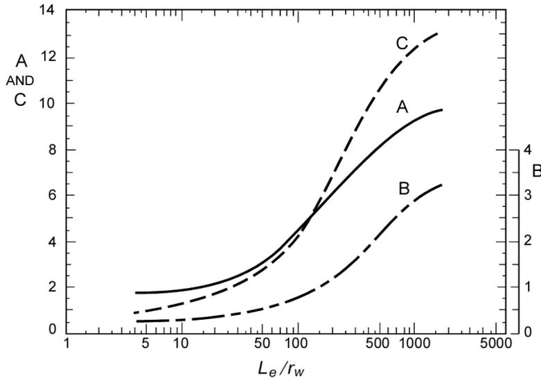
Figure 15.20 Dimensionless parameters A, B, and C as a function of  $L_e/r_w$  for calculation of  $\ln(R_e/r_w)$  in the Bouwer and Rice slug test. Bouwer, H., 1989: The Bouwer and Rice slug test. *Ground Water*, 27(3), p. 304-309. Reprinted by permission of Ground Water Publishing Company. Copyright 1989. All rights reserved.
