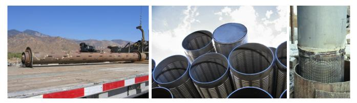
Figure 16.20 Common types of screens for high-capacity production wells. *Left*: Slotted casing, photo courtesy of Adrian Ezeagy. *Middle*: Shutter type screen, photo courtesy of Adrian Ezeagy. *Right*: Continuous slot wire-wound stainless-steel screen (often referred to as Johnson screen) welded to the riser pipe and being lowered into a newly drilled well.
