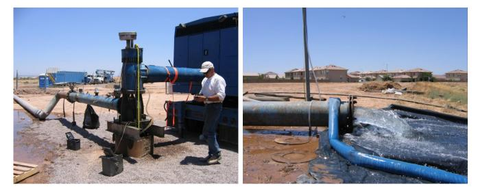
Figure 15.37 Large capacity deep production well in Arizona being tested with the maximum feasible pumping rate. Tests like this produce large quantities of water which must be managed for extended period of time, including preventing the water to circle back to the aquifer and bias the test results. Photos courtesy of Chris Legg.
