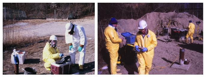
Figure 14.1 Use of personal protective equipment (PPE) during sampling of groundwater impacted by volatile organic compounds (left), and setup for an aquifer pumping test (right) by hydrogeologist Roger Pennifill and his crew of Ebasco Environmental, Inc. at Mattiace Petrochemical Superfund site, Glen Cove, New York.
