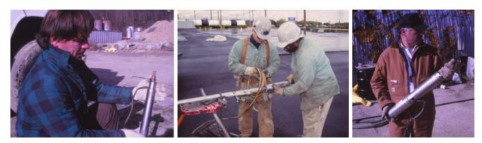
Figure 16.26 Submersible well pumps come in many different sizes and capacity, from gallons per minute to tens of gallons per minute (shown on the photos), and as powerful as hundreds of gallons per minute or more, with the lift of hundreds of feet or more.
