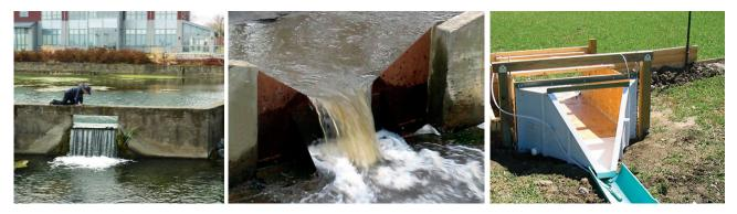
Figure 15.11 *Left*: Rectangular weir measuring outflow from a spring in Winchester, Virginia formerly utilized for public water supply. *Middle*: Sharp-crested 120 degrees V-notch weir. *Right*: Prefabricated H flume. Two right photographs courtesy of Don Meals, Tetra Tech, Inc., from NNPSMP, 2008; in public domain.
