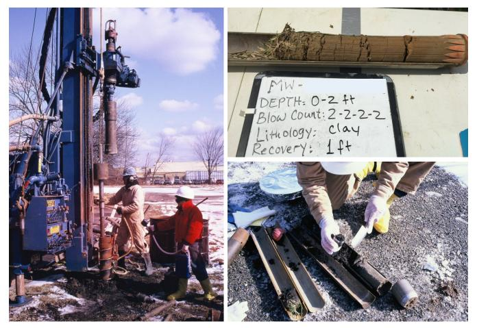
Figure 14.9 *Left*: Driving (hammering) split-spoon sampler through hollow-stem auger. *Right*: soil samples are exposed after retrieving and splitting the sampler. Bottom right photo shows collection of hydrocarbon-contaminated soil sample for laboratory analysis. Top right photo courtesy of Dawit Yifru.
