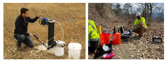
Figure 15.8 *Left*: Low-flow sampling equipment. Courtesy of *In-Situ* (https://in-situ.com/us/low-flow-sampling). *Right*: Low-flow sampling at a site in Pennsylvania, United States. Photo courtesy of Jeff Manuszak.
