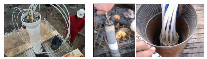
Figure 14.25 Examples of commercially available multi-level monitoring systems. *Left photo*: FLUTe, Flexible Liner Underground Technologies (https://www.flut.com/). *Two right photos*: single-casing Multilevel Groundwater Monitoring System CMT by Solinst (https://www.solinst.com/products/multilevel-systems-and-remediation/). All photos courtesy of Peter Thompson.
