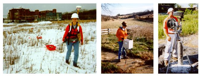
Figure 14.4 *Left*: Surveying with Geometrics Ohm mapper capacitively coupled resistivity meter. *Middle*: Scintrex CG-3M microgravity meter. *Right*: Borehole video inspection setup. Photos courtesy of Timothy Bechtel.
