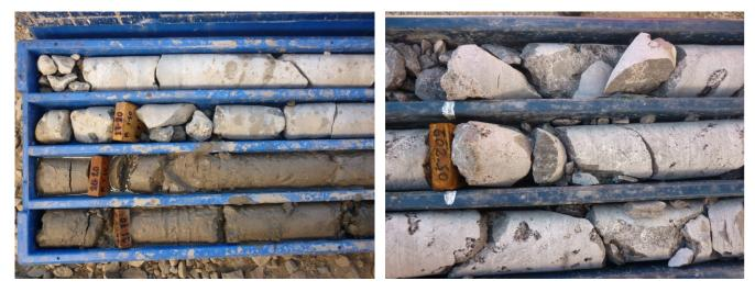
Figure 14.16 Dolomitic rock core from an exploration boring at a site in Peruvian Andes. *Left:* Upper, highly weathered portion of bedrock with a clay-filled cavity. *Right:* Broken-up core in highly fractured and karstified (vuggy) section of bedrock at ~600 meters (1,970 feet) below ground surface.
