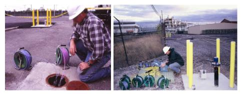
Figure 15.27 Hydrogeologist Andy Clark setting up a system for continuous monitoring of multiple monitoring wells at the startup of a pump-and-treat groundwater remediation at a site in New England. Cables from pressure transducers at the wells converge on the central datalogger.
