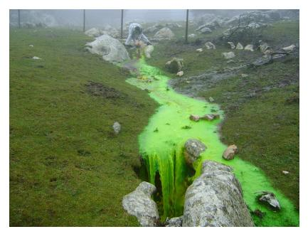
Figure 5.34 Dye tracing test with uranine in the karst system of Alta Cadena range near Malaga, Spain. Courtesy of Bartolome Andre Navarro, CEHIUMA.
