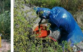
Figure 15.39 Left: Injection of Rhodamine WT into a water-level observation well. Photo courtesy of Charles J. Taylor, USGS. *Right*: Dilution of sodium fluoresceine prepared for dye tracing experiment in karst. Dilution of powdered tracer is with water, but use of NaOH and/or alcohol may accelerate the process. Courtesy of Zoran Stevanović.
